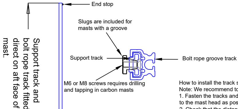
On masts with groove the support track and solid ramp is fastened with slugs
